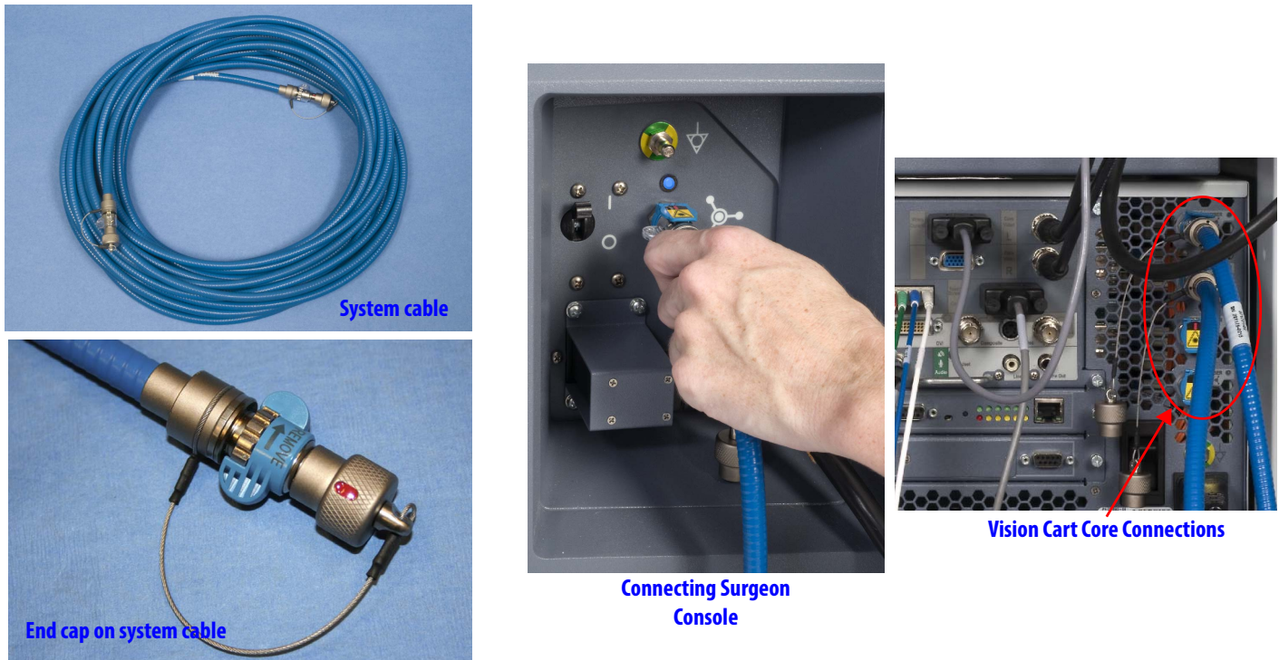
Figure 4.1 Sample system cable and connections
