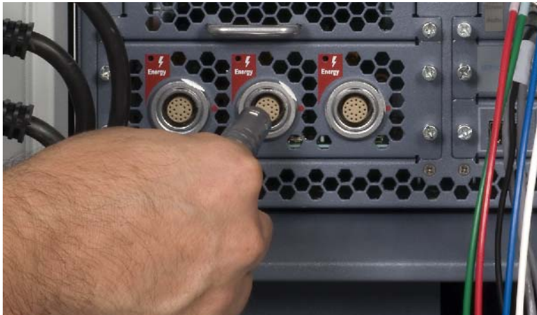
Figure 4.14 Auxiliary device connections (back of Core)
