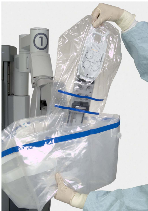
Figure 6.9 Lowering the drape over the insertion axis
