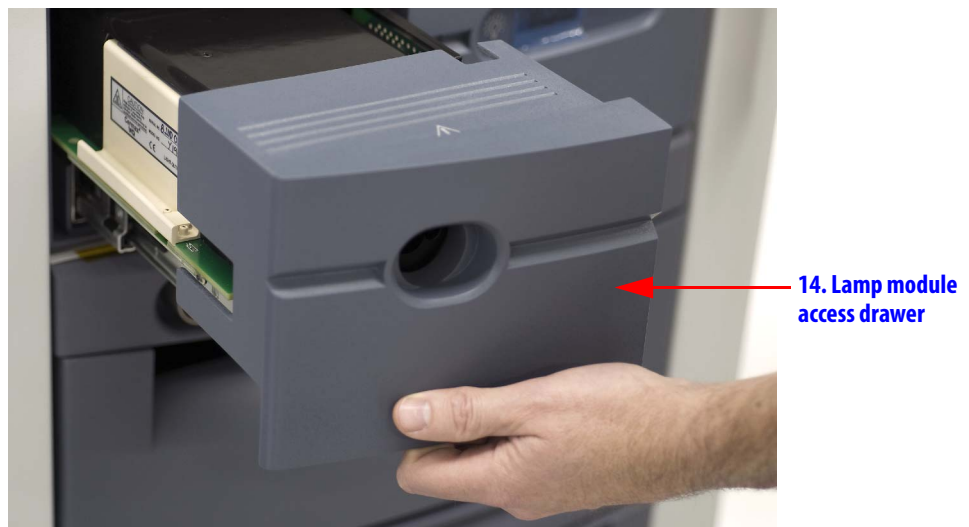
Figure C.5 Lamp module access drawer open
