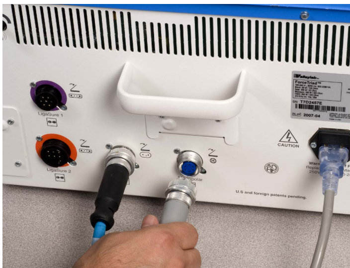
Figure 4.13 Auxiliary device connection (back of ESU)
