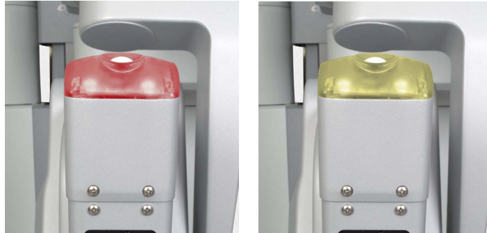
Figure A.2 Arm LEDs in fault states
