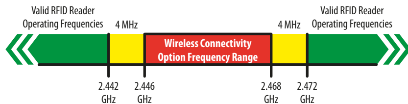
Figure 6 Valid RFID Reader Operating Frequencies
