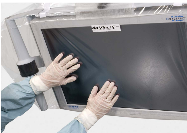
Figure 6.27 Smoothing the drape on the monitor
