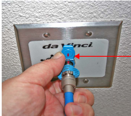
Figure D.6 Connect other end of fiber cable to fiber wall plate
