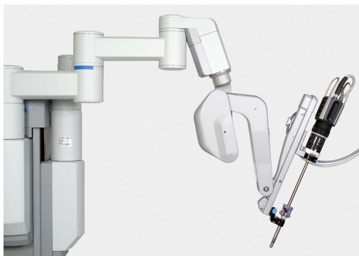
Figure 2.14 Camera arm with attached endoscope
