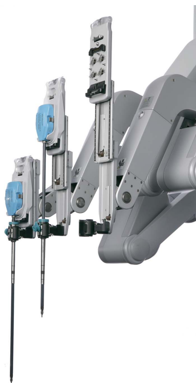
Figure 9.1 Instruments installed on the insertion axes
