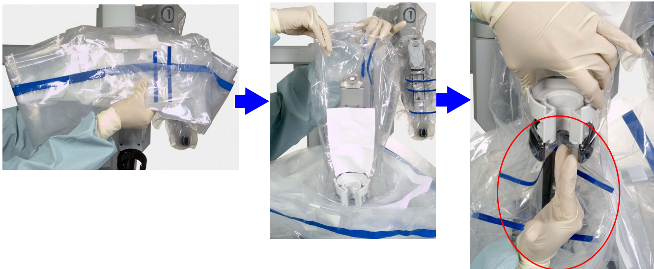
Figure 6.16 Lower over insertion axis, install sterile adapter
