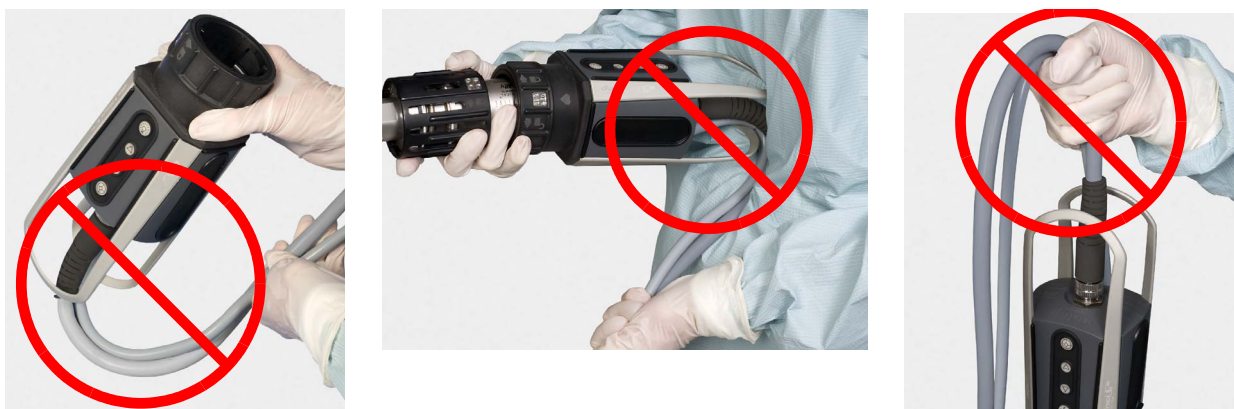
Figure 7.4 Examples of mishandling camera head cables
