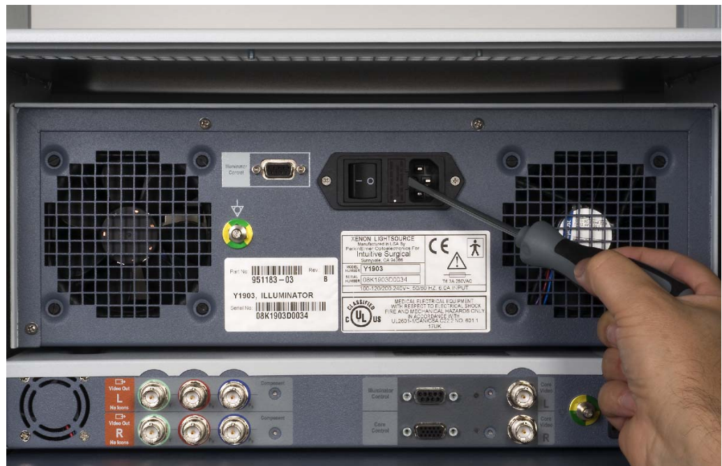
Figure C.6 Remove fuse cover
