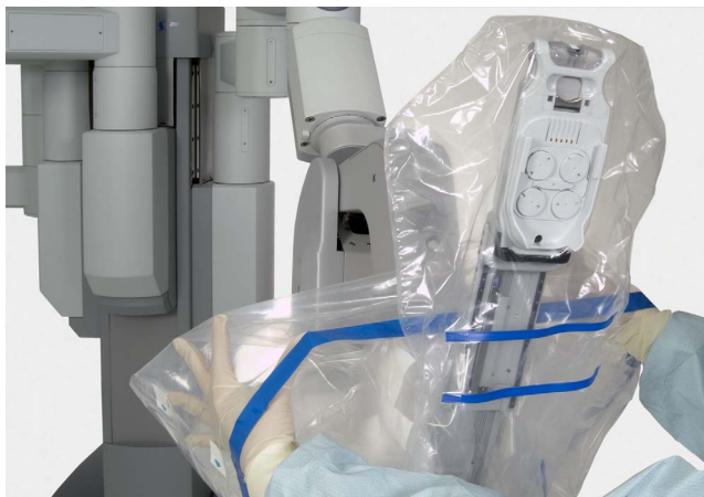
Figure 6.11 Stretching the drape along the arm
