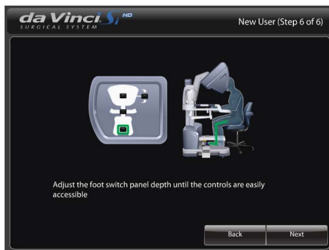
Step 6: Adjust foot switch panel depth
