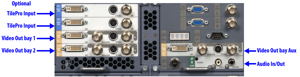
Figure H.1 Video and audio connections (back of Core)
